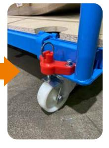
The steering locks are mounted on the transport device and, when actuated, the castor is fixed in the direction of travel by activating a pin with a bayonet lock. With this locking, swivel castors with run-on plates become fixed castors with good tracking and the transported goods glide smoothly.
