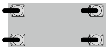
Four swivel castors, if necessary, a swivel castor with a directional lock can be used.
