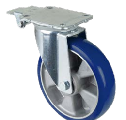
Central locking device in the castor Locking of the swivel head and wheel rotation without changing the position of the brake. Possibility of central locking of up to 4 castors.
